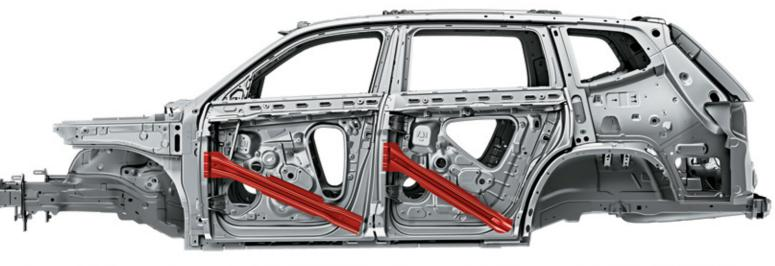
Front and rear crumple zones help absorb crash energy, while a rigid safety cage helps deflect it away from the driver and passengers.
